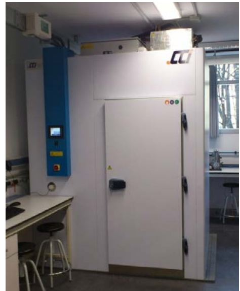
Figure 2 Climatic chamber used for MBV tests
