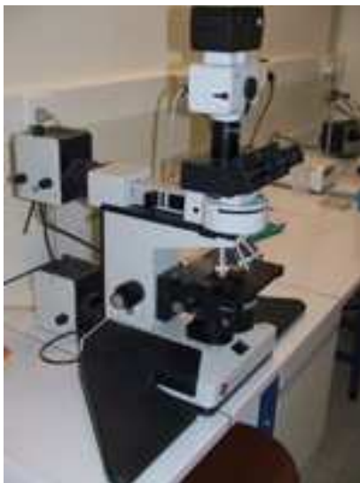
Figure 4. Epifluorescence microscope and image of a sample stained with acridine orange.
