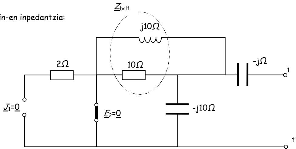
$$Z_{\text{bal}1} = \frac{j10 \cdot 10}{10 + j10} = \frac{j100}{10\sqrt{2} \angle 45^\circ} = 5\sqrt{2} \angle 45^\circ = (5 + j5)\Omega$$
