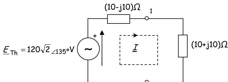
$$\underline{I} = \frac{120\sqrt{2} \angle 135^\circ}{20} = 6\sqrt{2} \angle 135^\circ A \quad \text{eta potentzia: } \hat{P} = 10 \cdot (6\sqrt{2})^2 = 720W$$
