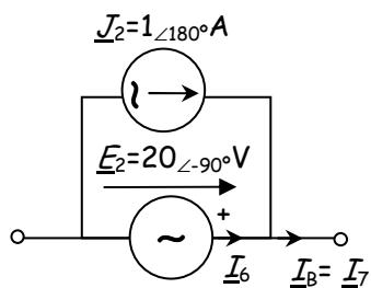
$$\underline{I}_6 = \underline{I}_B - \underline{J}_2 = -2 + j + 1 = (-1 + j) = \sqrt{2} \angle 135^\circ A$$
