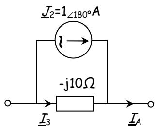
$$\underline{I}_3 = \underline{I}_A - \underline{J}_2 = (1 + j) A = \sqrt{2} \angle 45^\circ A$$
