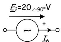
$$\underline{S}_{E2} = \underline{E}_2 \cdot \underline{I}_6^* = (-j20)(-1 - j) = (-20 + j20) \text{ VA} = -(20 - j20) \text{ VA}$$
