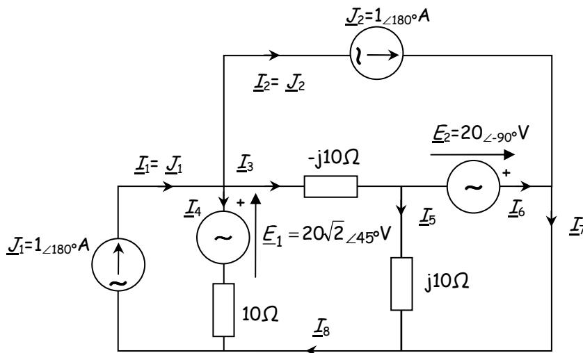
$$\underline{I}_1 = \underline{J}_1 + \underline{0} = 1 \angle 180^\circ + \underline{0} = 1 \angle 180^\circ A$$
