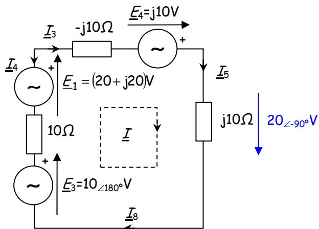
$$\underline{I}_8 = \frac{20\angle -90^\circ + 10\angle 180^\circ + 20\sqrt{2}\angle 45^\circ + 10\angle 90^\circ}{10 - j10} = \frac{-j20 - 10 + 20 + j20 + j10}{10 - j10} = \frac{10 + j10}{10 - j10} =$$
