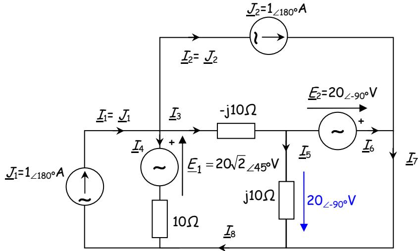
$$\underline{I}_5 = \frac{-20\angle -90^\circ}{10\angle 90^\circ} = -2\angle 180^\circ = 2\angle 0^\circ A$$
