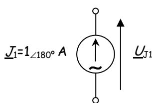
$$\underline{U}_{J1} = 10 \underline{I}_4 + \underline{E}_1 = -10 - j10 + (20 + j20) = (10 + j10) \text{ V} = 10\sqrt{2} \angle 45^\circ \text{V}$$
