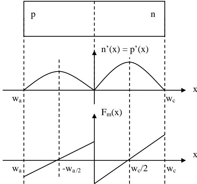
$$p'_n(x) = \frac{G_L}{2D_p} \cdot x(w_c - x); \quad F_{p-n}(x) = G_L \cdot \left( x - \frac{w_c}{2} \right)$$
