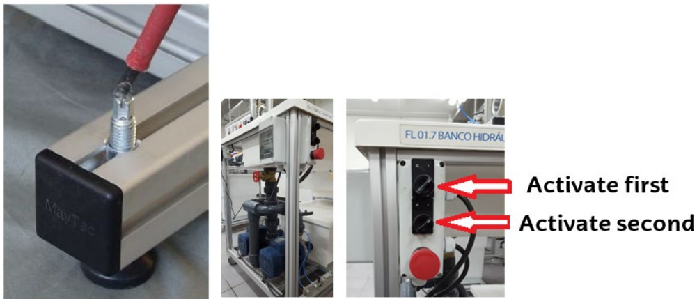
Figure 27: Levelling system of the turbine and switches for the activation of the pumps.
