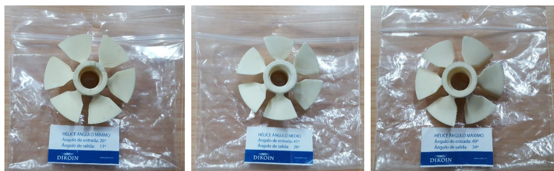
Figure 24: Different types of runners available to work with the Kaplan turbine.
