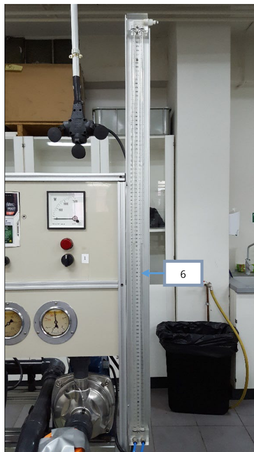
Figure 4: Graduated columns (6) connected to an orifice plate.
