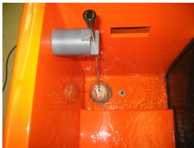
Figure 15. Drainage ball valve.
