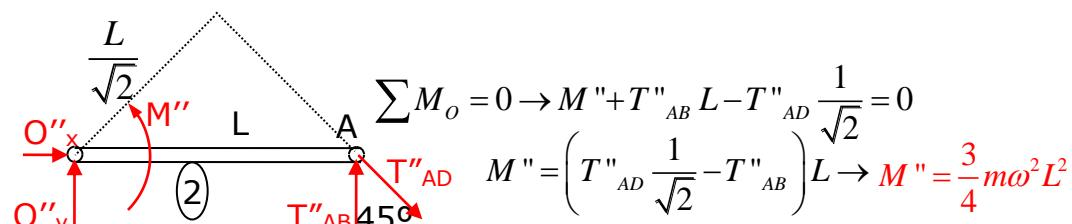
GAINJARPENA:  $\vec{M} = \vec{M}' + \vec{M}'' = \left( \frac{PL}{2} + \frac{3}{4}m\omega^2 L^2 \right) \vec{k}$
