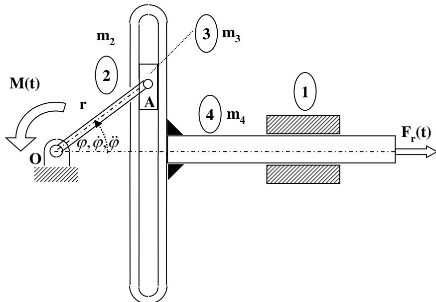
$$M_m(t) - F_r(t)r \sin \varphi = I_O \ddot{\varphi} + m_3 r^2 \ddot{\varphi} + m_4 r^2 \sin \varphi (\dot{\varphi} \sin \varphi + \dot{\varphi}^2 \cos \varphi)$$
