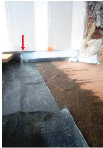
Photo 5: Construction opening with a temporary stud wall wrapped with polyethylene sheet to create an air seal during the test.
