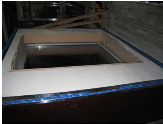
Figure 2a. calibration setup for measuring extraneous air leakage of the setup. Figure 2b. Installation of aluminum window frame and wood reveal.
