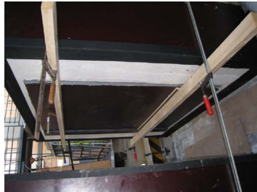
Figure 2a. calibration setup for measuring extraneous air leakage of the setup. Figure 2b. Installation of aluminum window frame and wood reveal.
