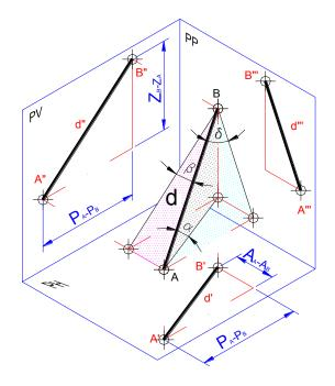
The angle between the segment and the projection planes PH, PV and PP can also be calculated by constructing these triangles. The angle between the segment and the projection plane PH is calculated using d'. The angle between the segment and the projection plane PV is calculated using d'' and the one formed with PP is calculated making use of d'''.
