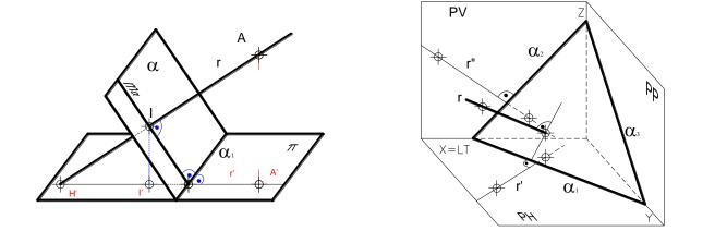
As it has been said before, if a line is perpendicular to a plane, the projections of the line are perpendicular to the homonymous traces of the plane: **r**' is perpendicular to  $\alpha_1$  and **r**'' is perpendicular to  $\alpha_2$ .
