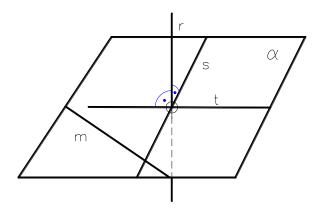
From the previous statement it can be concluded that in order to check the orthogonality of a line and a plane, it is enough if the line is perpendicular to two non-parallel lines in the plane or to two non-parallel lines that are parallel to the plane. If a line is perpendicular to a plane, it is perpendicular to all lines in the plane.
