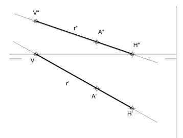
The lines that are parallel to the planes XY and XZ have only one trace, because one of its two projections is parallel to the floor-line (LT).
