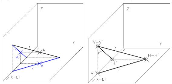
The intersections of the line with the projection planes (PH and PV) are called traces.
