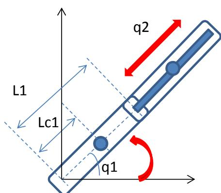
$${}^{i-1}A = \begin{bmatrix} C\theta_i & -C\alpha_i S\theta_i & S\alpha_i S\theta_i & \alpha_i C\theta_i \\ S\theta_i & C\alpha_i C\theta_i & -S\alpha_i C\theta_i & \alpha_i S\theta_i \\ 0 & S\alpha_i & C\alpha_i & d_i \\ 0 & 0 & 0 & 1 \end{bmatrix}$$
