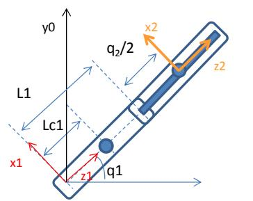
$${}^0_2 A = {}^0_1 A {}^1_2 A = \begin{bmatrix} -Sq & 1 & 0 & Cq & 1 & \boxed{Cq(1(L_1 + \frac{q_2}{2}))} \\ Cq & 1 & 0 & Sq & 1 & \boxed{Sq(1(L_1 + \frac{q_2}{2}))} \\ 0 & 1 & 0 & 0 & 0 & \\ 0 & 0 & 0 & 1 & 1 & \end{bmatrix} = \begin{array}{l} x \\ y \\ z \end{array}$$
