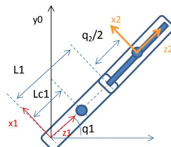
$$K_2 = \frac{1}{2} m_2 \left[ \dot{q}_1^2 (L_1 + q_2/2)^2 + \dot{q}_2^2 - 2\dot{q}_1\dot{q}_2(L_1 + q_2/2)S(q_1/2) \right] + \frac{1}{2} I_2 \dot{q}_1^2$$
