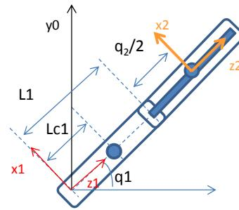
$$J = \begin{bmatrix} \frac{\partial x}{\partial q_1} & \frac{\partial x}{\partial q_2} & \frac{\partial x}{\partial q_3} \\ \frac{\partial y}{\partial q_1} & \frac{\partial y}{\partial q_2} & \frac{\partial y}{\partial q_3} \\ \frac{\partial z}{\partial q_1} & \frac{\partial z}{\partial q_2} & \frac{\partial z}{\partial q_3} \end{bmatrix} = \begin{bmatrix} -Sq_1(L_1 + q_2/2) & Cq_1/2 & 0 \\ Cq_1(L_1 + q_2/2) & Sq_1/2 & 0 \\ 0 & 0 & 0 \end{bmatrix}$$
