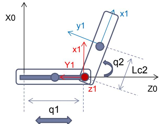
$$J = \begin{bmatrix} \frac{\partial x}{\partial q_1} & \frac{\partial x}{\partial q_2} & \frac{\partial x}{\partial q_3} \\ \frac{\partial y}{\partial q_1} & \frac{\partial y}{\partial q_2} & \frac{\partial y}{\partial q_3} \\ \frac{\partial z}{\partial q_1} & \frac{\partial z}{\partial q_2} & \frac{\partial z}{\partial q_3} \end{bmatrix} = \begin{bmatrix} 0 & L_{c2}Cq_2 & 0 \\ 0 & 0 & 0 \\ 1 & -L_{c2}Sq_2 & 0 \end{bmatrix}$$
