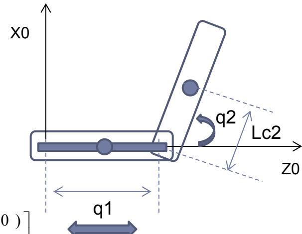
$${}^0_2 A = {}^0_1 A {}^1_2 A = \begin{bmatrix} C(q_2 - 90) & 0 & 0 & L_{c2}C(q_2 - 90) \\ 0 & -1 & 0 & 0 \\ -S(q_2 - 90) & 0 & -1 & -L_{c2}S(q_2 - 90) + q_1 \\ 0 & 0 & 0 & 1 \end{bmatrix} \rightarrow \begin{aligned} x &= L_{c2}C(q_2 - 90) = L_{c2}Sq_2 \\ y &= 0 \\ z &= -L_{c2}S(q_2 - 90) + q_1 = L_{c2}Cq_2 + q_1 \end{aligned}$$
