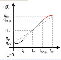
$$q_{III}(t_{fin}) = q_{fin} = a_{III} + b_{III} t_{fin} + c_{III} t_{fin}^{2}$$
