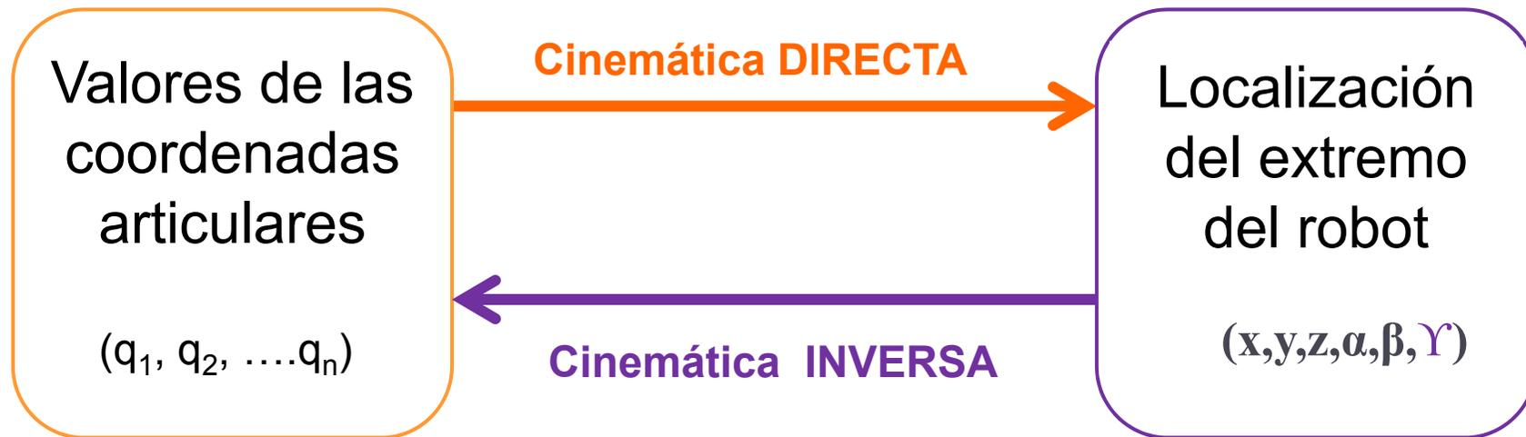
$$\begin{aligned}x &= f_x(q_1, q_2, \dots, q_n) \\y &= f_y(q_1, q_2, \dots, q_n) \\&\dots\dots\dots \\ \Upsilon &= f_\Upsilon(q_1, q_2, \dots, q_n)\end{aligned}$$
