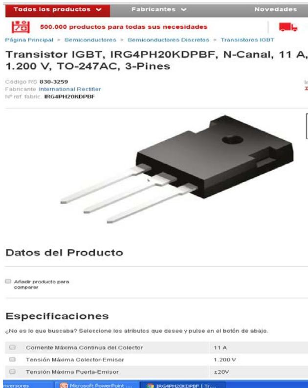
Transistor IGBT, IRG4PH20KDPBF, N-Canal, 11 A, 1.200 V, TO-247AC, 3-Pines
