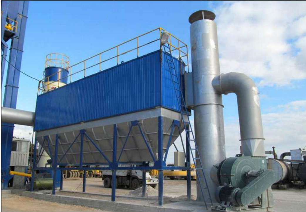
“Baghouse dust collector for asphalt plants” by Cornhorn licensed under CC BY-SA 3.0
