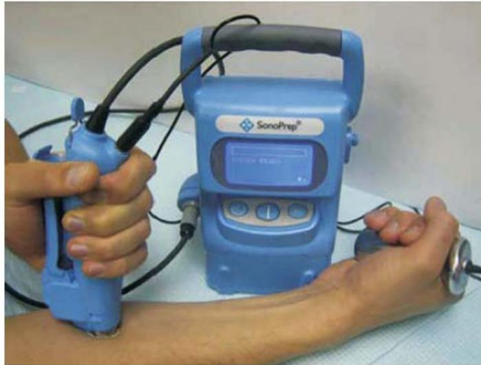
**Figure 4. Low-frequency ultrasound treatment in a clinical setting with the SonoPrep<sup>®</sup> device (Echo Therapeutics, Franklin, MA, USA). The patient holds a conductive polymer hand-piece and the device automatically stops when the skin impedance is decreased to the desired treatment level. Usual treatment times are on the order of 10 s (reprinted with permission from [92]).**
