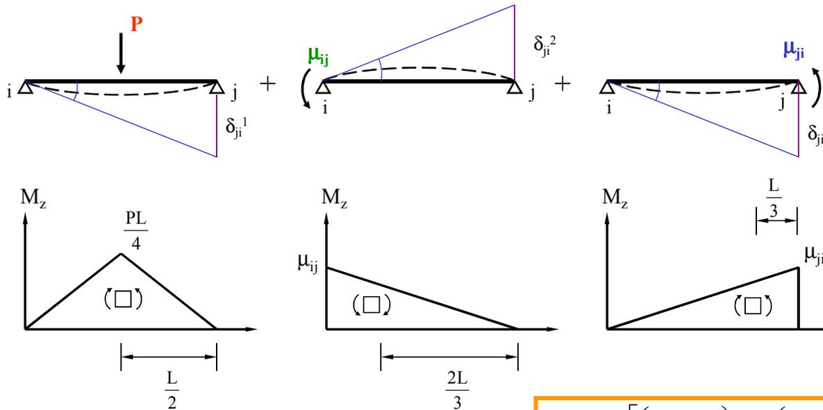
$$\theta_i = \theta_i^{(P)} - \theta_i^{(\mu_{ij})} + \theta_i^{(\mu_{ji})} = \frac{\delta_{ji}^1 - \delta_{ji}^2 + \delta_{ji}^3}{L} \Rightarrow \theta_i = \frac{1}{EI} \left[ \left( \frac{1}{2} L \frac{PL}{4} \right) \frac{L}{2} - \left( \frac{1}{2} L \mu_{ij} \right) \frac{2L}{3} + \left( \frac{1}{2} L \mu_{ji} \right) \frac{L}{3} \right] = \frac{1}{EI} \left[ \frac{PL^2}{16} - \frac{\mu_{ij}L}{3} + \frac{\mu_{ji}L}{6} \right] = 0 \quad (a)$$
