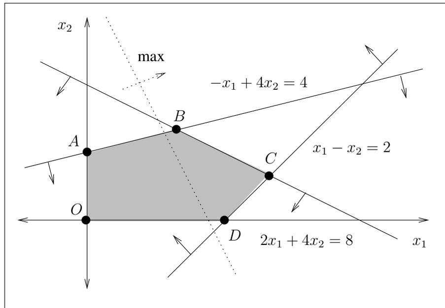
The polygon  $OABCD$  is a convex set. The extreme-points in the convex set can be determined by solving linear equations systems.
