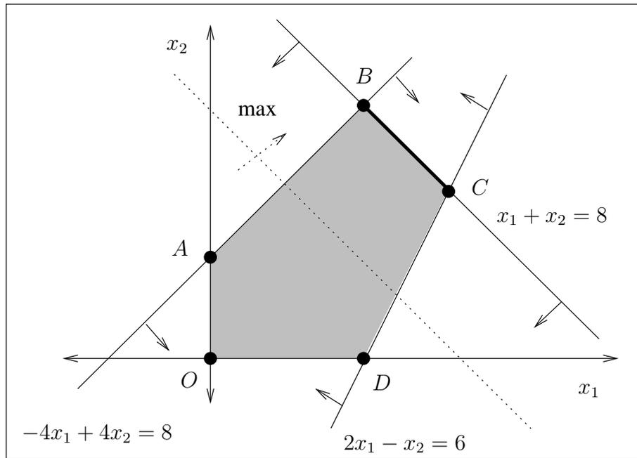
$z$  increases as we move the objective function line in a northeast direction, so the largest value of  $z$  in the feasible region occurs at some points on the boundary of the region. Extreme-points  $B$  and  $C$ , together with all points on the line segment  $BC$  are optimal. The optimal objective function value is  $z^* = 8$ .
