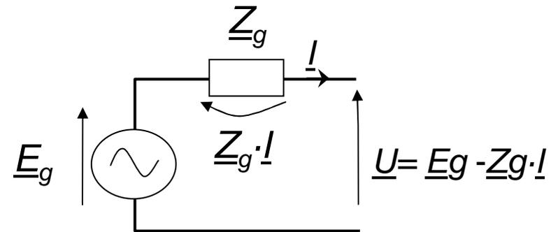
$$\underline{S} = \underline{U} \cdot \underline{I}^* = S_{\angle\varphi^\circ} = P + jQ \quad \underline{S}_g = \underline{E}_g \cdot \underline{I}^* = S_g \angle\varphi^\circ = P_g + jQ$$
