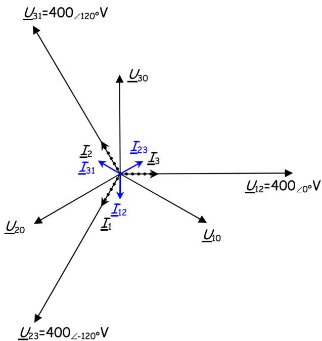
$$\underline{I}_{12} = \frac{400 \angle 0^\circ}{15 \angle 90^\circ} = \left[ \frac{80}{3} \right] \angle -90^\circ A$$
