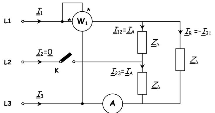
$$\underline{I}_A = \frac{U_{13}}{30 \angle 90^\circ} = \frac{400 \angle -60^\circ}{30 \angle 90^\circ} = \left[ \frac{200}{15} \right] \angle -150^\circ, \quad \underline{I}_B = \frac{U_{13}}{15 \angle 90^\circ} = \frac{400 \angle -60^\circ}{15 \angle 90^\circ} = \left[ \frac{400}{15} \right] \angle -150^\circ$$
