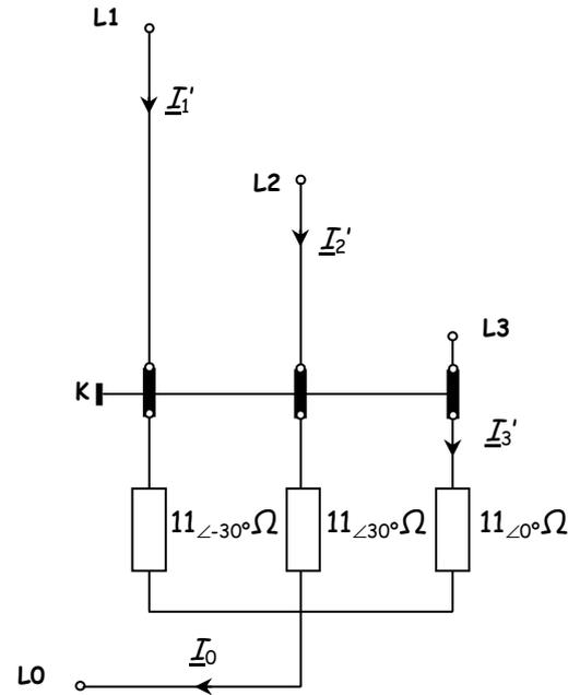
$$\underline{I}_0 = \underline{I}_1' + \underline{I}_2' + \underline{I}_3' = 20 \angle 60^\circ + 20 \angle 120^\circ + 20 \angle -90^\circ = j(20\sqrt{3} - 20) \text{ A} = 14,64 \angle 90^\circ \text{ A}$$
