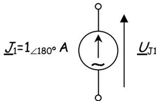
$$\underline{U}_{J1} = 10\underline{I}_4 + \underline{E}_1 = -10 - j10 + (20 + j20) = (10 + j10) \text{ V} = 10\sqrt{2} \angle 45^\circ \text{ V}$$
