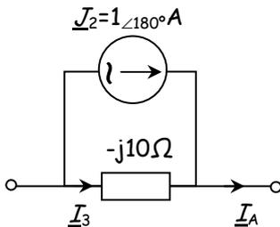
$$\underline{I}_3 = \underline{I}_A - \underline{J}_2 = (1 + j) \text{ A} = \sqrt{2} \angle 45^\circ \text{ A}$$
