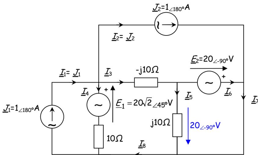
$$\underline{I}_5 = \frac{-20 \angle -90^\circ}{10 \angle 90^\circ} = -2 \angle 180^\circ = 2 \angle 0^\circ \text{ A}$$
