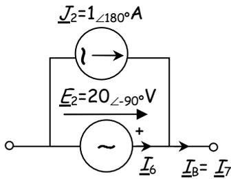
$$\underline{I}_6 = \underline{I}_B - \underline{J}_2 = -2 + j + 1 = (-1 + j) = \sqrt{2} \angle 135^\circ \text{ A}$$
