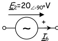
$$\underline{S}_{E2} = \underline{E}_2 \cdot \underline{I}_6^* = (-j20)(-1 - j) = (-20 + j20) \text{ VA} = -(20 - j20) \text{ VA}$$
