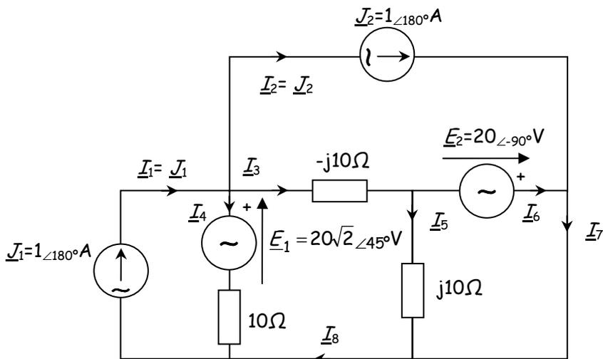
$$\underline{I}_1 = \underline{J}_1 + \underline{0} = 1 \angle 180^\circ + 0 = 1 \angle 180^\circ \text{ A}$$
