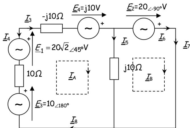
$$E_1 = 10 \cdot 1 \angle 180^\circ = 10 \angle 180^\circ \text{ V}$$
