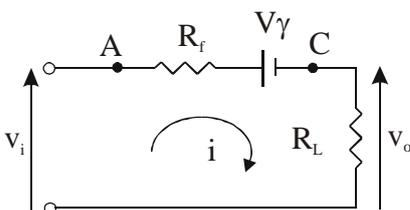
$$i = \frac{v_i - V_\gamma}{R_f + R_L}$$
